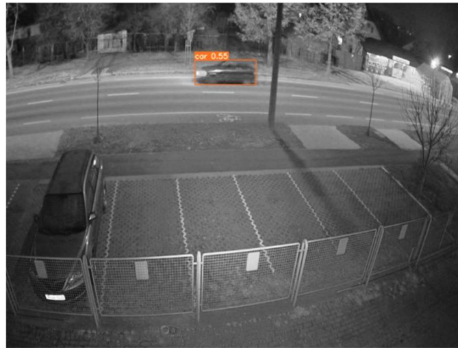
Figure 1. The road section on the camera image at night. The object identified as a car is in the orange bounding box.
